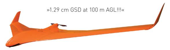
The **BRAMOR UAS** is based on a blended wing body modular airframe, with the emphasis on the smallest possible T/O weight, advanced aerodynamics, electric propulsion, endurance, ergonomic and user friendly ground control station, robust fail-safe systems and procedures, durability and mobility.
